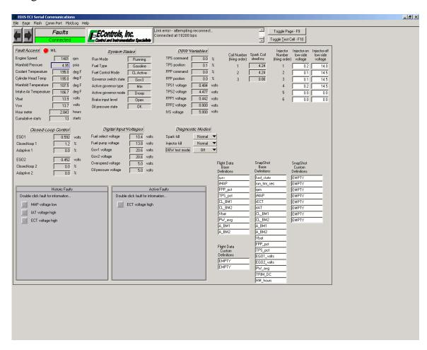
The System Fault screen is used to view and clear DTC's, which have been set.
